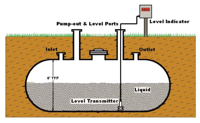
As these tanks fill with the hydrocarbon condensate a reliable level indication is required to indicate when the tank reaches a predetermined level.
